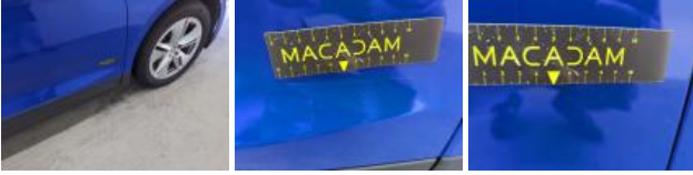
Door FR, Scratch(es), Repair and paint (complete)
