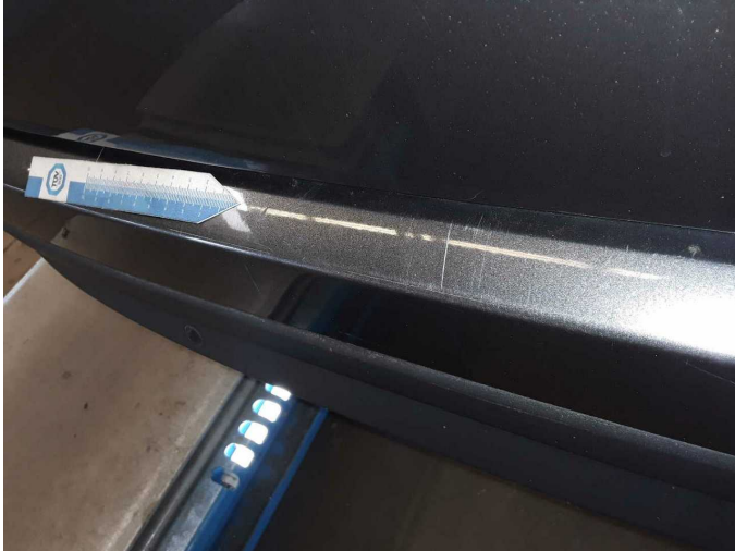
Damage 7: Rear bumper: Rear bumper - Scratch(es) - Paint
