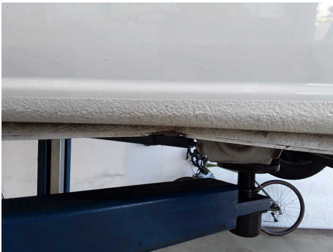
Damage 4: Sill - left side: Sill - Deformed - Repair and paint
