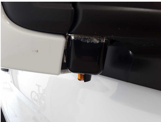
Damage 2: Indicator - front: Mirror - right side (Kappe fehlt) - Differs from the original configuration - Replace
