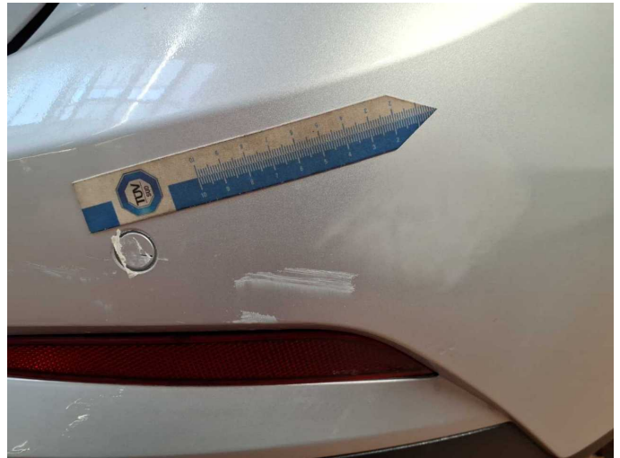
Damage 1: Rear bumper: Rear bumper (inkl. Parksensoren) - Scratch(es) - Paint
