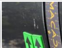
Door FL, Dent(s) and scratch(es), Acceptable
