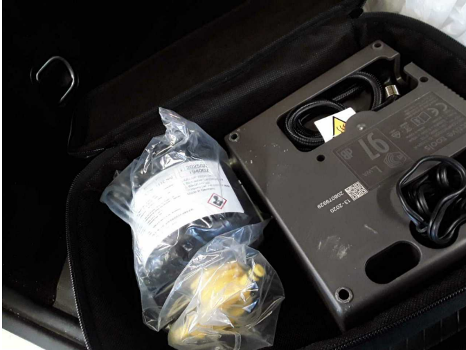
Damage 2: Equipment: Tirefit filler - Expired - Replace
