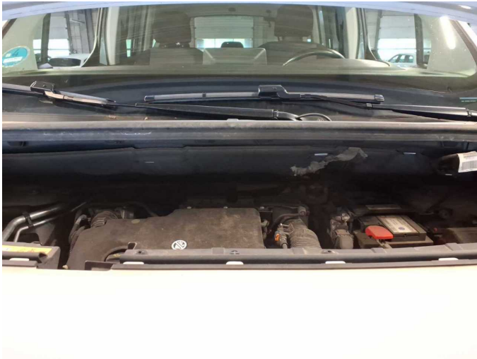
Damage 5: Misc.: Misc. (Dämmung Stirnwand) - Damage caused by marten / rodent - Replace
