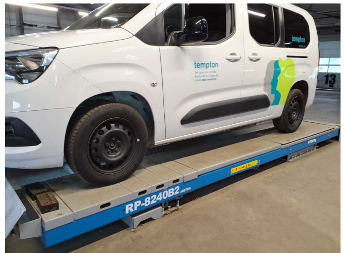
Damage 15: Wheel / tyres: Tyres - complete set (Stahl statt Alufelgen) - Differs from the original configuration - Replace
