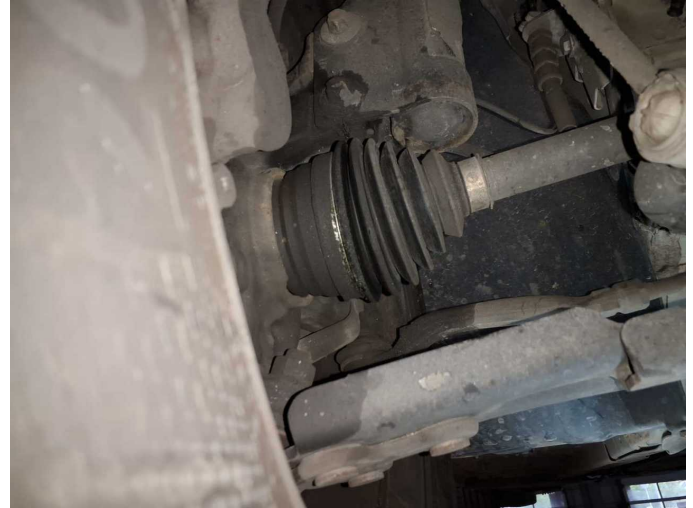
Damage 10: Drive train: Sleeve prop shaft - front right side - Broken / torn - Replace
