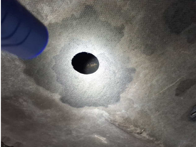
Damage 7: Engine: Engine - Leaking - Perform diagnosis
