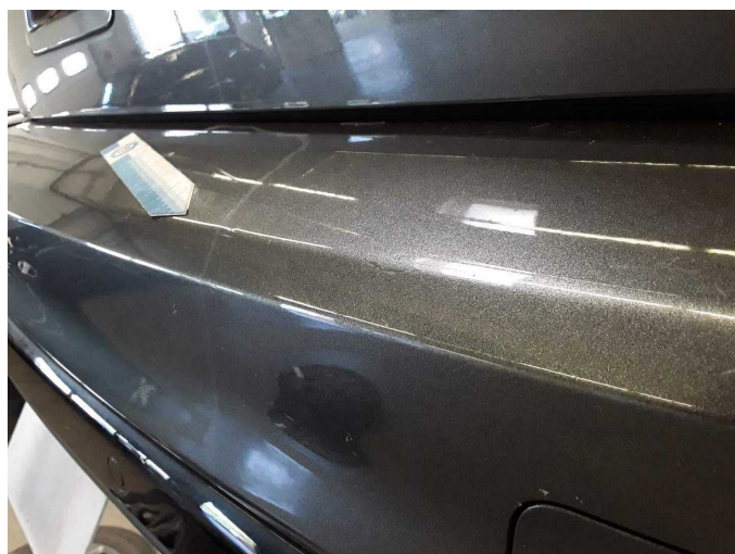
Damage 3: Rear bumper: Rear bumper - Scratch(es) - Paint
