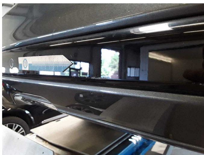
Damage 3: Rear bumper: Rear bumper - Scratch(es) - Paint
