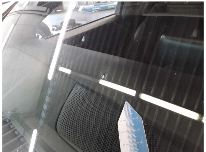
Damage 7: Vehicle glazing: Windscreen - Stone chips - Replace
