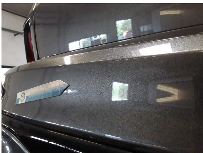
Damage 3: Rear bumper: Rear bumper - Scratch(es) - Paint
