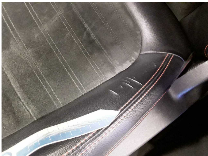
Damage 2: Seat - front: Seat cover - left side - Porous / cracked - Smart repair
