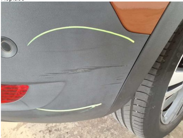
Damage #13: Rear bumper: Spoiler - Scratched - Replace
