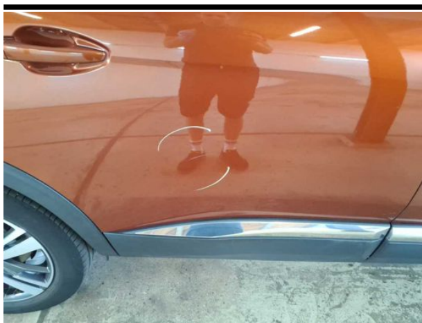
Beschädigung #10: Tür hinten rechts: Tür - Delle / Lackschaden - Smart Repair
