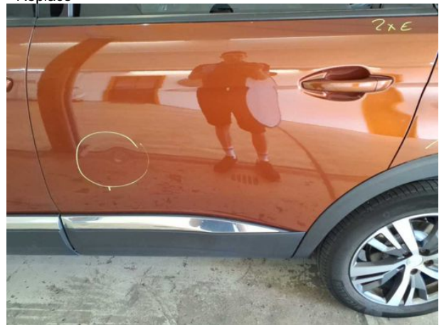
Damage #14: Door - rear left side: Door - Dent / paintcoat damage - Repair and paint
