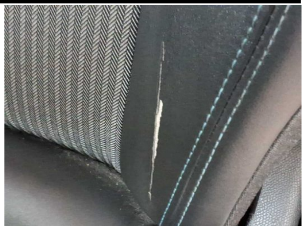
Damage #12: Seat - front: Backrest cover - left side - Damag... - Replace
