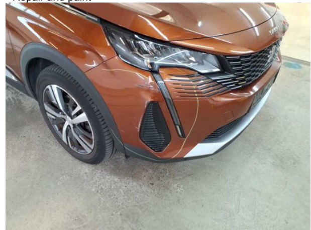
Damage #16: Front bumper: Front bumper - Scratched - Replace
