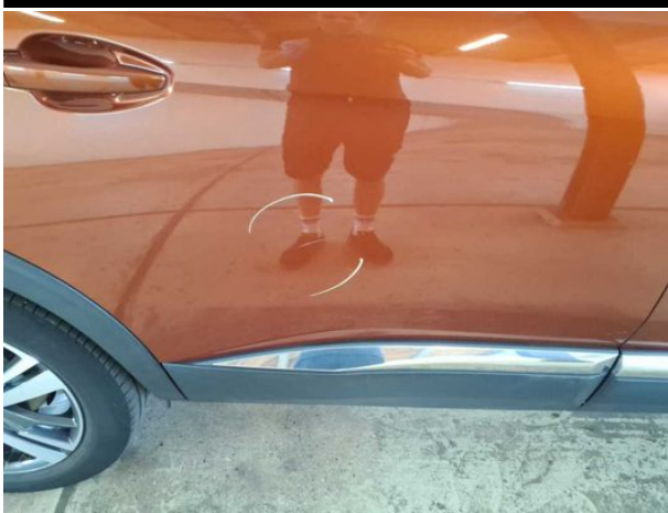
Damage #10: Door - rear right side: Door - Dent / paintcoat damage - Smart repair
