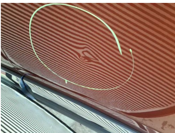
Damage #14: Door - rear left side: Door - Dent / paintcoat damag... Repair and paint
