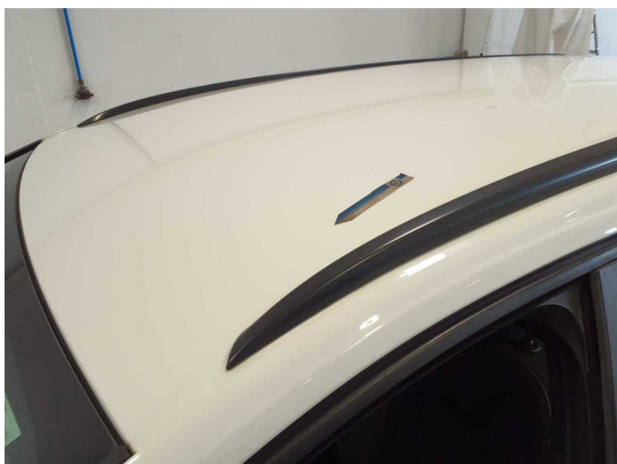
Damage 14: Roof: Roof - Dent / paintcoat damage - Paint
