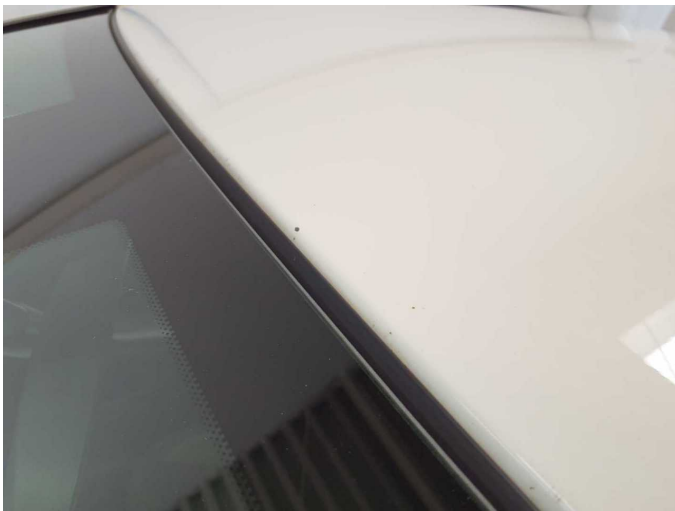
Damage 14: Roof: Roof - Dent / paintcoat damage - Paint
