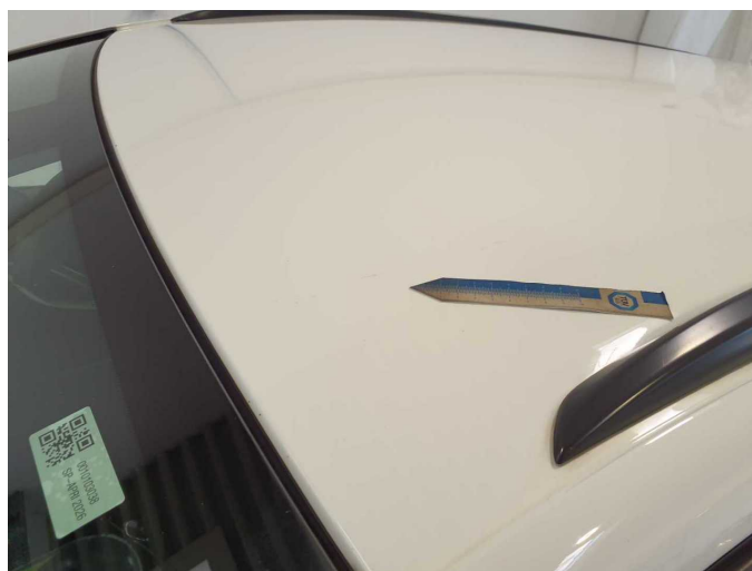
Damage 14: Roof: Roof - Dent / paintcoat damage - Paint
