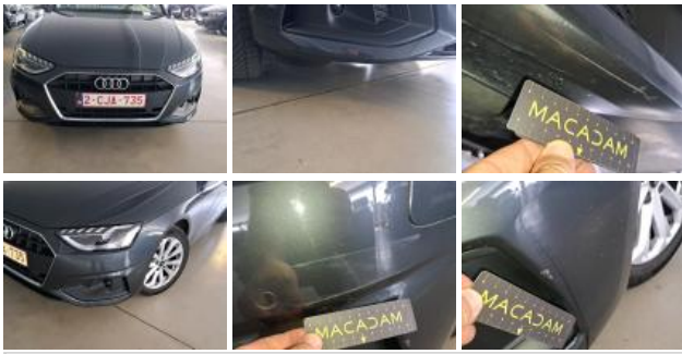
Door FL, Dent(s) and scratch(es), Acceptable
