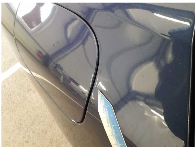
Damage 2: Side panel - rear right side: Side panel (Lackläufer) - Paint defect - Paint
