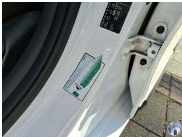
2. Türeinstieg Vorne - Links Delle - Smart Repair
