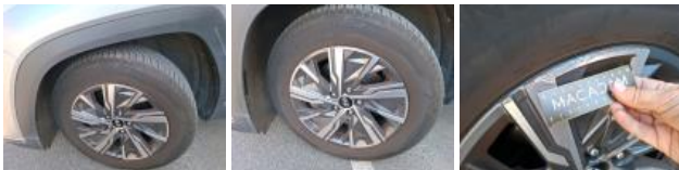
Tyre RL, Out of tolerance, Replace
