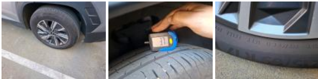
Tyre RR, Out of tolerance, Replace
