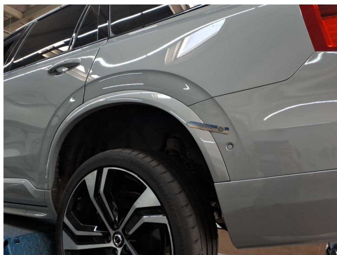
Wear and tear 3: Side panel - rear left side: Wheel well extension - Scratch(es) - No deduction
