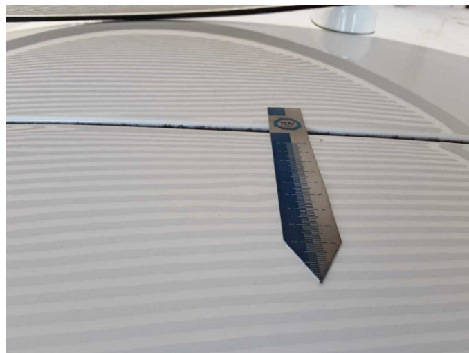
Damage 6: Boot lid / rear door: Rear spoiler - dent(s) - Repair and paint
