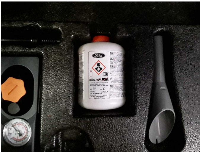
Damage 2: Equipment: Tirefit filler - Expired - Replace
