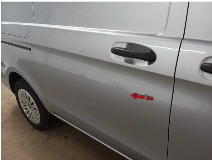
Damage 4: Sliding door, right: Sliding door - dent(s) - Repair and paint
