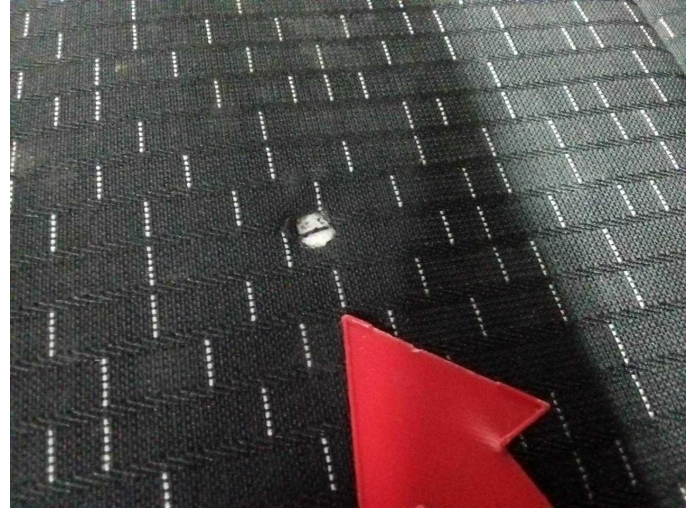
Damage 3: Seat - front: Seat cover - left side - Holes - Replace
