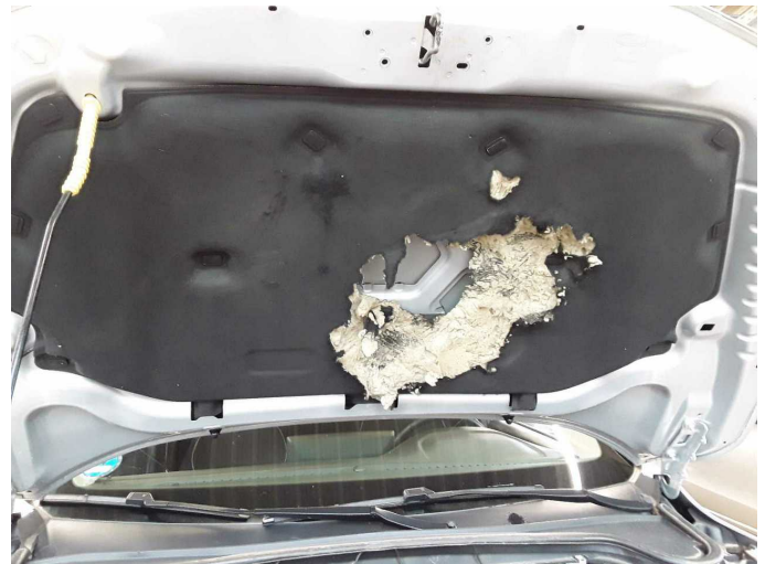
Damage 1: Bonnet: Insulation lining - Damage caused by marten / rodent - Replace
