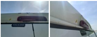
Roof reinforcement R, Dent(s) and scratch(es), Repair and paint (complete)
