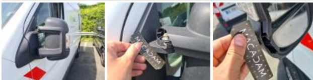
Side repeater L, Broken, Replace
