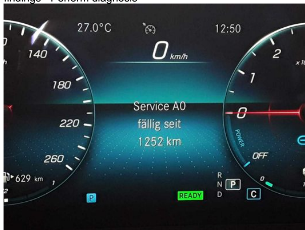
Damage #5: Misc.: Inspection / maintenance - Due - Replace
