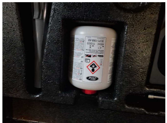
Damage 3: Equipment: Tirefit filler - Expired - Replace
