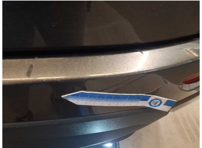
Damage 8: Rear bumper: Rear bumper - Scratched - Paint
