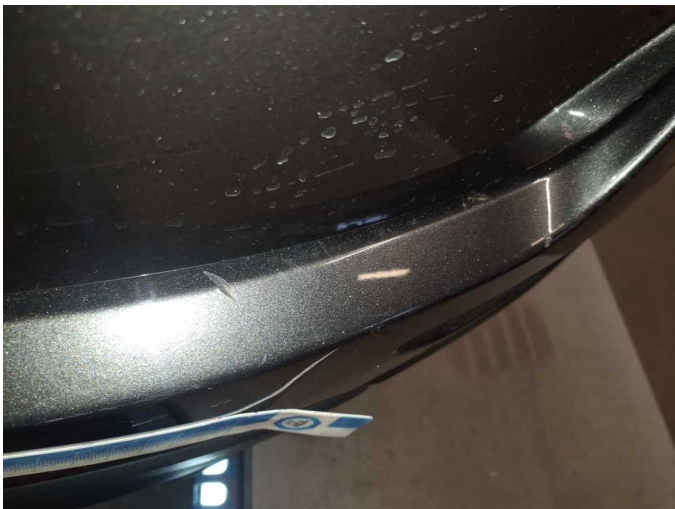
Damage 8: Rear bumper: Rear bumper - Scratched - Paint
