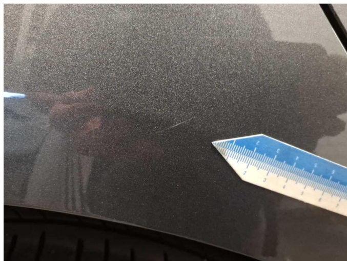
Wear and tear 3: Side panel - rear right side: Side panel (polierbar) - Scratch(es) - No deduction
