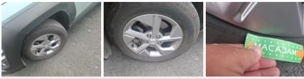
Tyre FR, Out of tolerance, Replace
