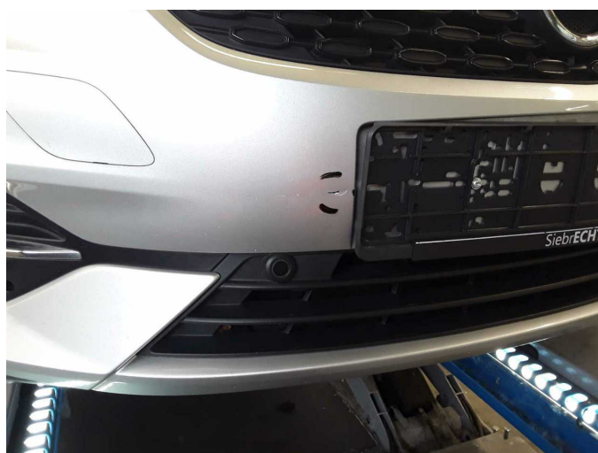
Damage 6: Front bumper: Front bumper - Scratch(es) - Paint
