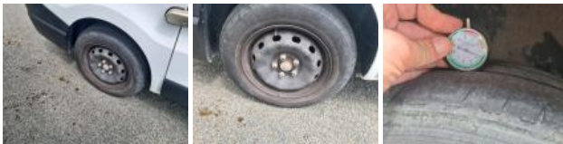
Wheel cover RR, Missing, Replace
