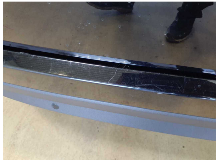
Damage 6: Rear bumper: Rear bumper - Scratch(es) - Paint
