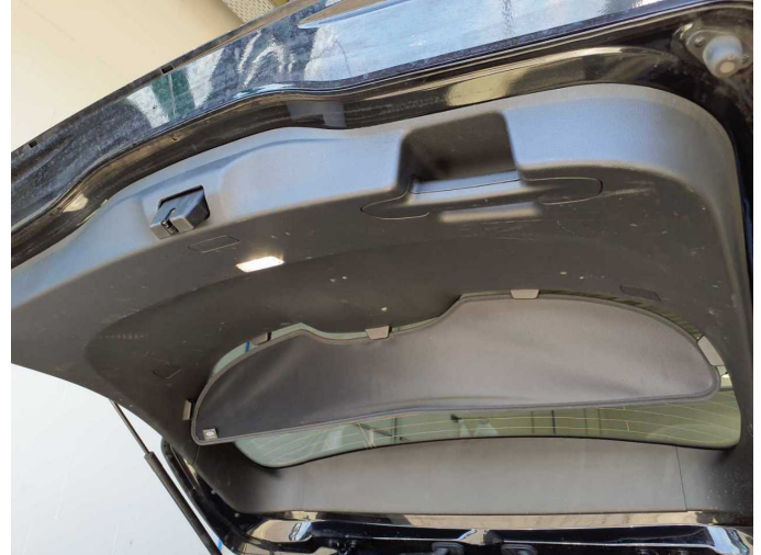
Damage 5: Trim / covers: Cargo area - lining - right side (+ links + Heckklappe) - Scratch(es) - Loss in value
