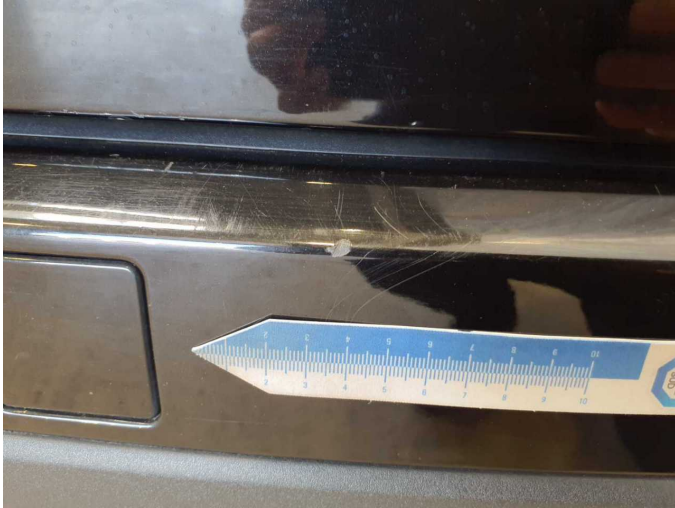
Damage 6: Rear bumper: Rear bumper - Scratch(es) - Paint
