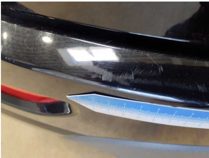
Damage 6: Rear bumper: Rear bumper - Scratch(es) - Paint
