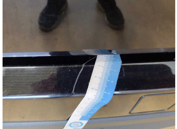
Damage 6: Rear bumper: Rear bumper - Scratch(es) - Paint
