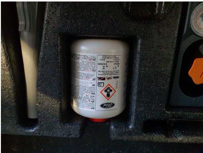
Damage 1: Equipment: Tirefit filler - Expired - Replace
