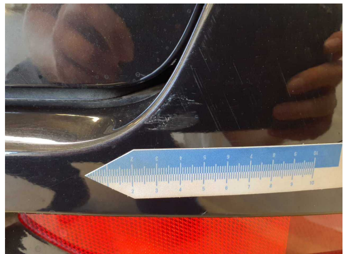
Damage 6: Rear bumper: Rear bumper - Scratch(es) - Paint
