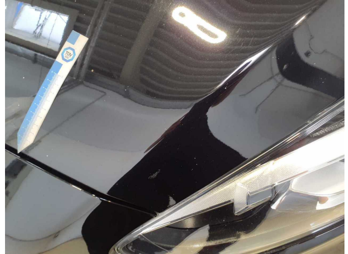
Damage 7: Bonnet: Bonnet - Stone chips - Paint
