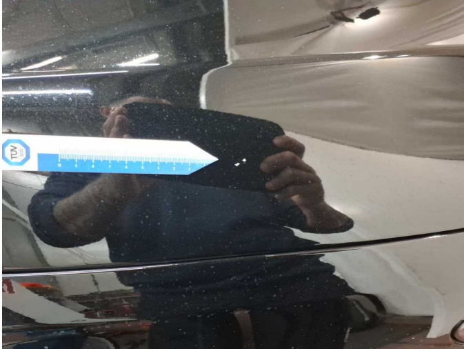
Damage 1: Bonnet: Bonnet - Stone chips - Smart repair
