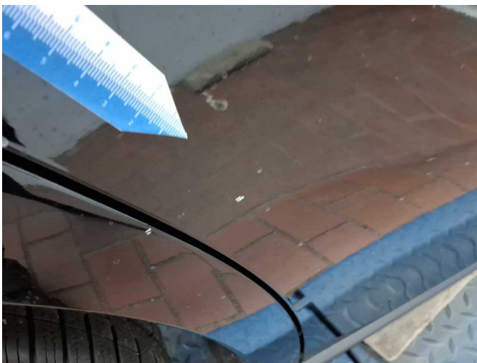
Damage 2: Door - rear right side: Door - Stone chips - Smart repair
