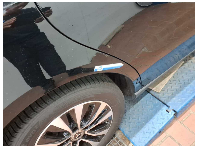
Damage 3: Side panel - rear right side: Side panel - Stone chips - Smart repair
