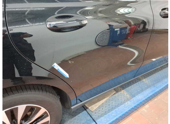
Damage 2: Door - rear right side: Door - Stone chips - Smart repair
