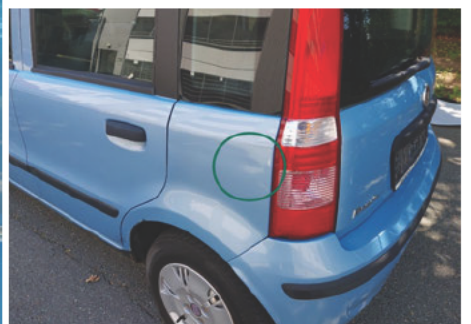
Kotflügel / Hinten Links / Delle
