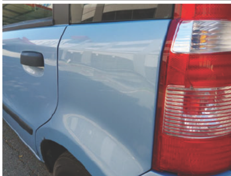
Kotflügel / Hinten Links / Delle
