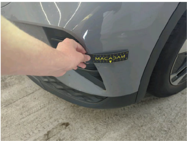
Bumper F Scratch(es) Repair and paint (complete) Front
