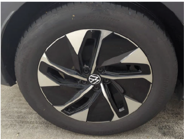
Alloy rim RR Scratch(es) Repair and paint (complete) Right
