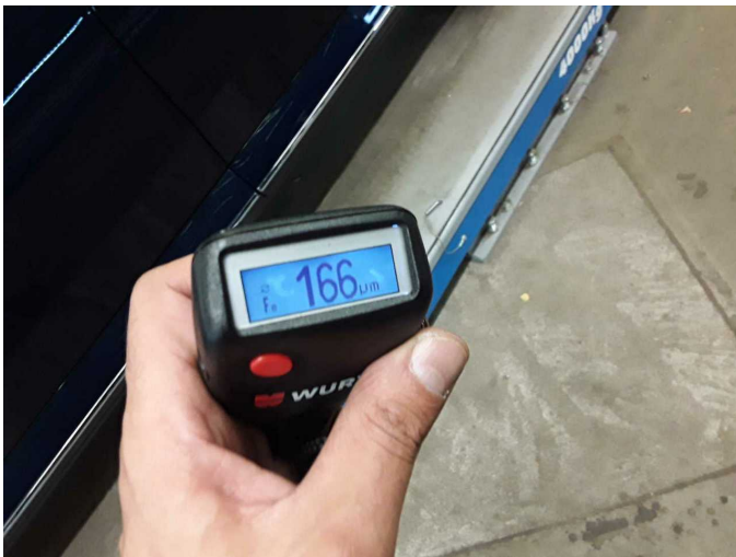
Repainting 1: Side panel - rear left side, Door - rear left side, Door - rear right side, Door - front right side
