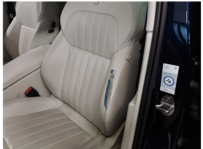
Damage 2: Seat - front: Backrest cover - left side - Worn - Smart repair
