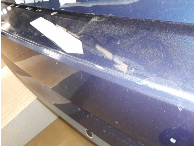
Damage 3: Rear bumper: Rear bumper (Verladebreich) - Scratch(es) - Smart repair
