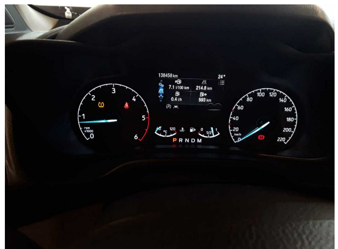
Damage 2: Wheel / tyres: Pressure sensor (Reifendruckkontrolle) - on - Perform diagnosis
