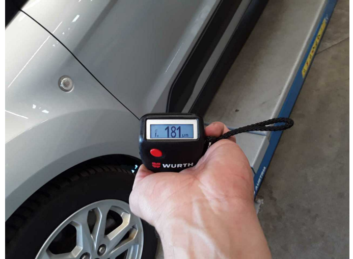
Repainting 1: Boot lid / rear door, Side panel - rear right side, Door - rear left side, Door - front left side
