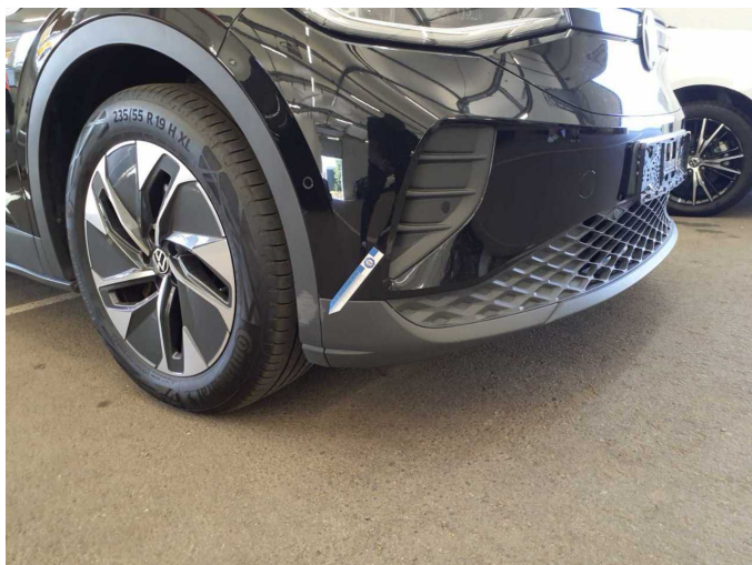
Damage 4: Front bumper: Spoiler - Scratch(es) - Replace
