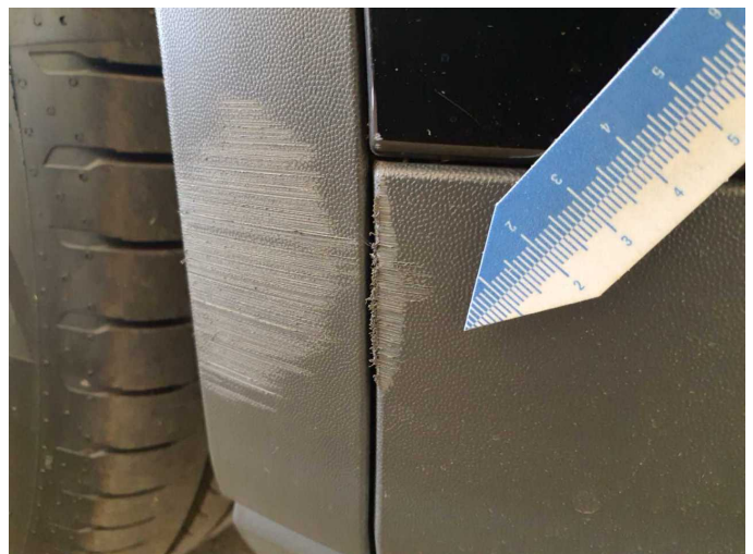
Damage 4: Front bumper: Spoiler - Scratch(es) - Replace
