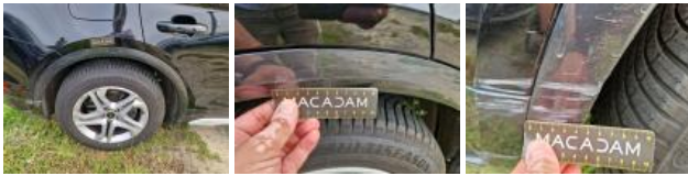
Wing RR, Dent(s), Repair and paint (complete)
