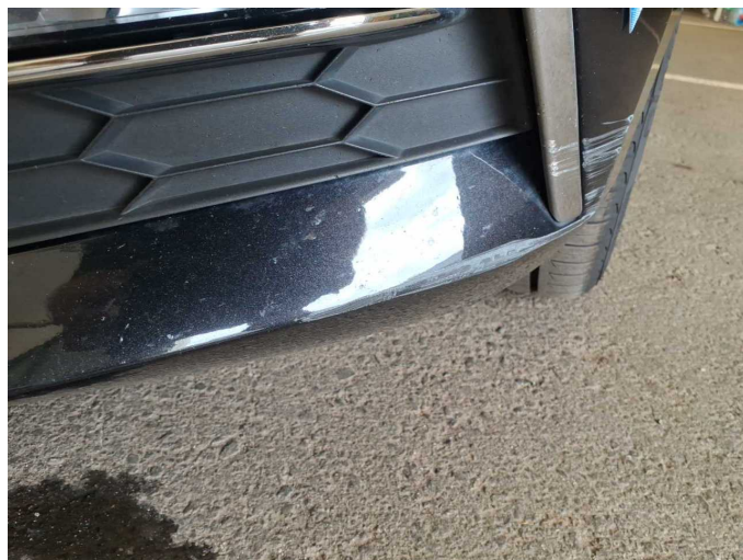
Damage 9: Front bumper: Front bumper (+ Blende) - Scratched - Paint
