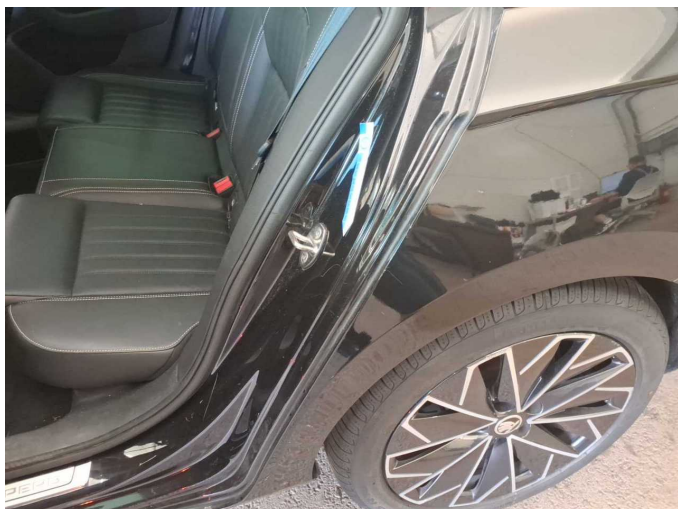
Damage 4: Side panel - rear left side: Side panel (Inkl. Einstieg) - Scratched - Smart repair
