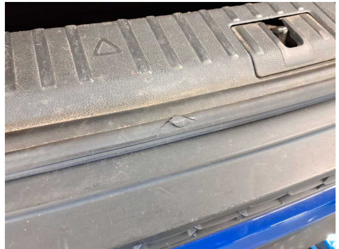
Damage 1: Boot lid / rear door: Seal - Broken / torn - Replace
