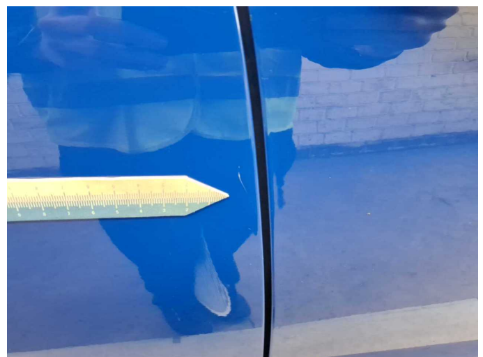
Damage 2: Door - rear right side: Door - Dent / paintcoat damage - Smart repair
