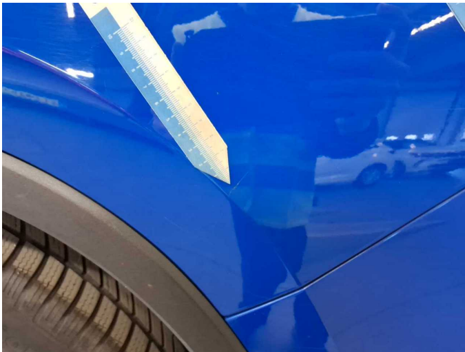
Damage 4: Side panel - rear left side: Side panel - Scratch(es) - Smart repair
