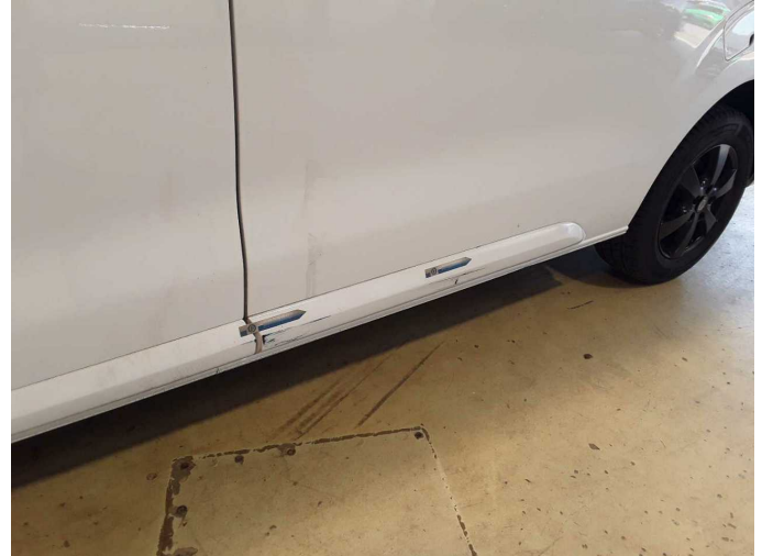
Damage 7: Door - front left side: Brightware - lower (+Tür hinten) - Damaged - Replace
