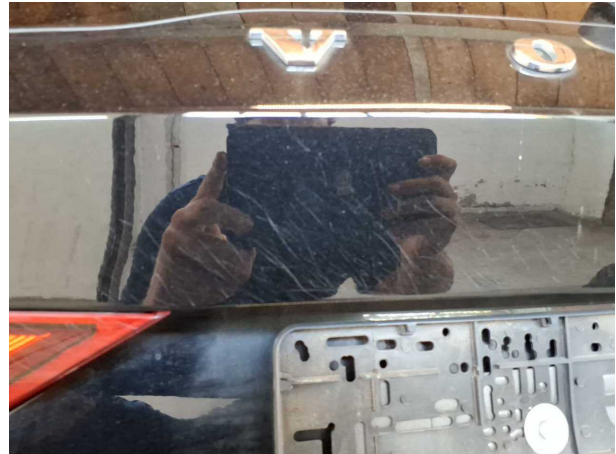
Damage #1: Boot lid / rear door: Boot lid - Scratched - Smart repair
