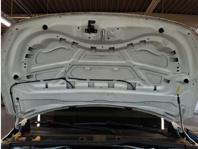
Damage 3: Bonnet: Insulation lining - Missing - Replace
