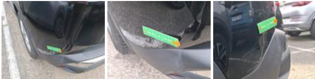
Bumper corner RL, Deformed / Strained, Repair and paint (complete)
