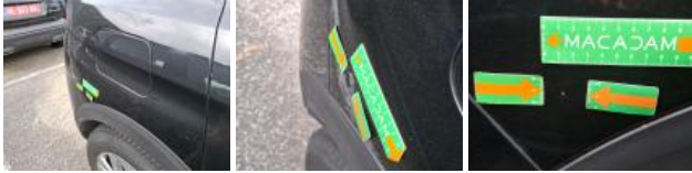
Door RR, Dent(s) and scratch(es), Repair and paint (complete)
