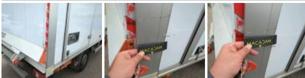
Shutter / cover R, Scratch(es), Replace
