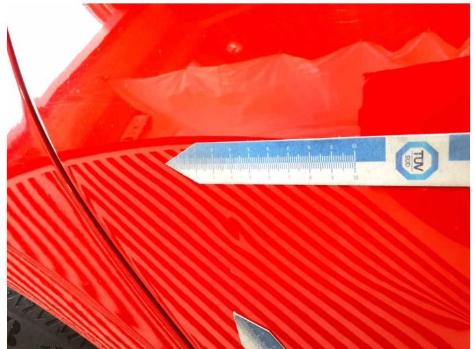
Damage 8: Door - rear right side: Door (Schleifspuren und Spachtel eingefallen) - Unprofessionally repaired - Repair and paint
