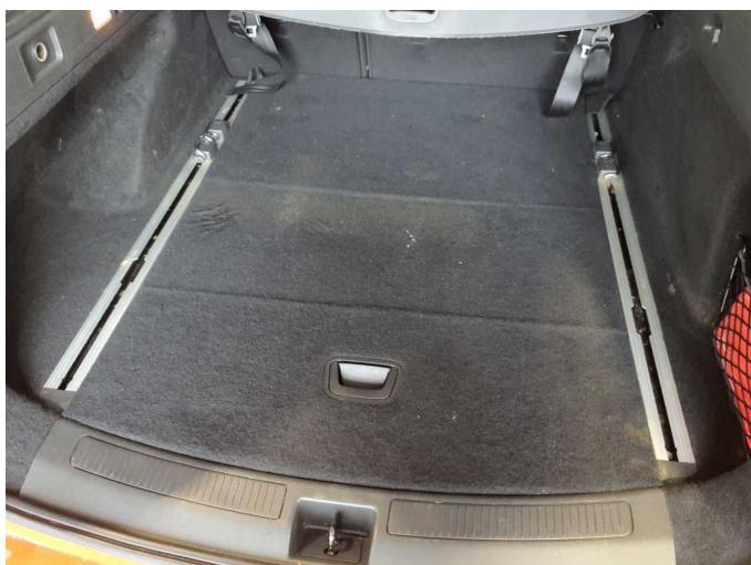
Damage 3: Interior: Cargo area floor (Griff) - Broken / torn - Replace
