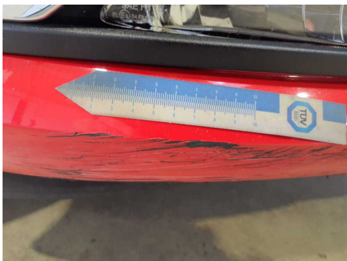
Damage 5: Front bumper: Front bumper - Scratch(es) - Paint
