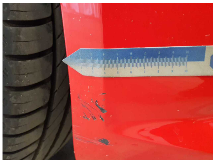
Damage 5: Front bumper: Front bumper - Scratch(es) - Paint
