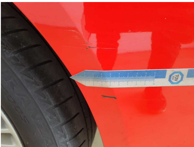
Damage 7: Rear bumper: Rear bumper - Scratch(es) - Paint
