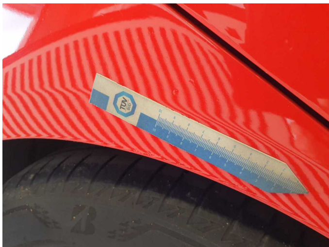
Damage 4: Side panel - rear right side: Side panel (Spachtelmasse eingefallen) - Unprofessionally repaired - Repair and paint
