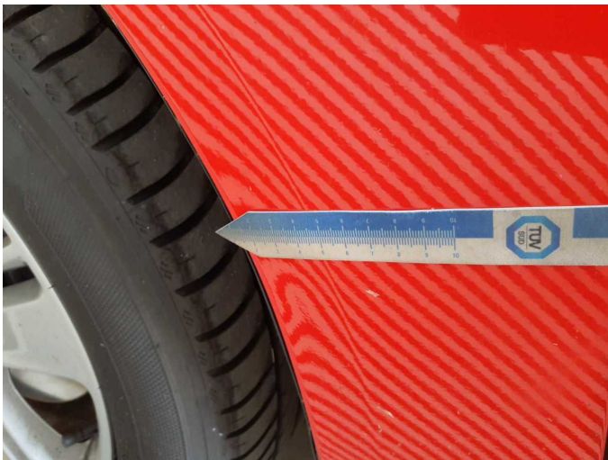
Wear and tear 7: Mudguard - left side: Mudguard - left side - dent(s) - No deduction
