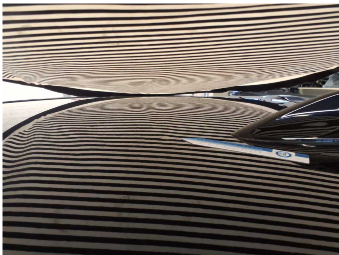
Damage 2: Roof: Roof - dent(s) - Smooth repair work
