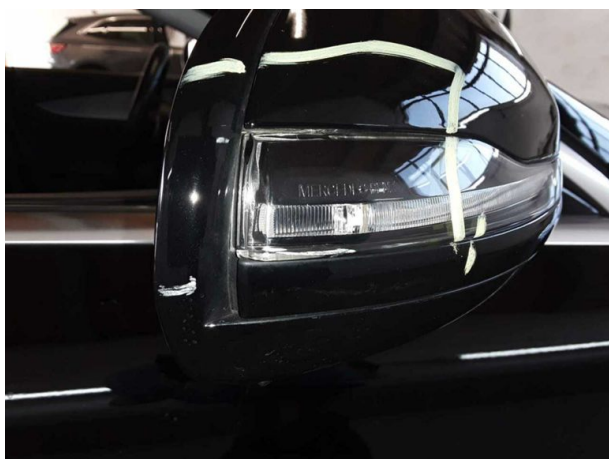
Damage #3: Indicator - front: Mirror - right side - Scratched - Replace
