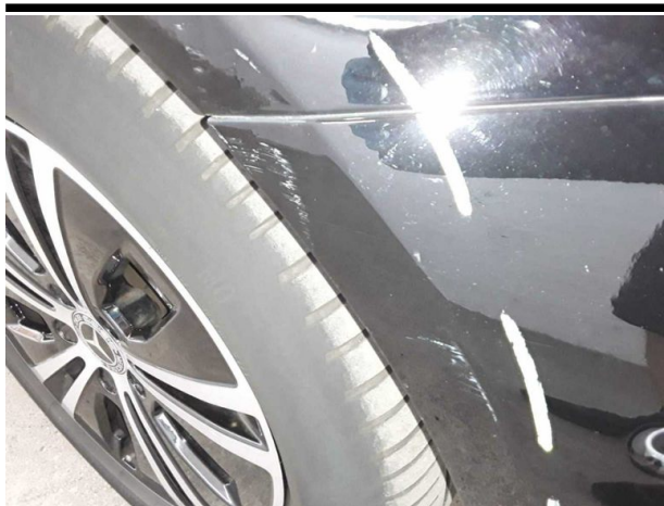
Damage #10: Front bumper: Bumper with Parktronic - Scratched - Repair and paint
