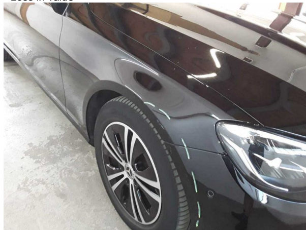
Damage #5: Mudguard - right side: Mudguard - right side - Scratched - Smart repair
