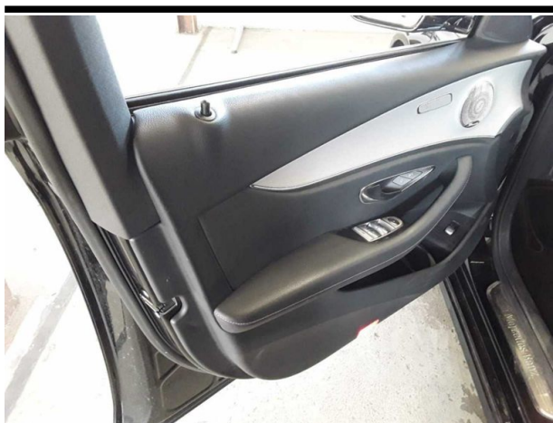
Damage #7: Trim / covers: Door trim - front left side - Damaged - Replace
