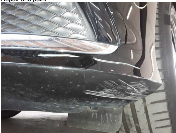
Damage #10: Front bumper: Bumper with Parktronic - Scratched - Repair and paint
