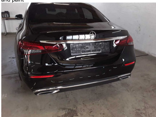
Damage #9: Rear bumper: Bumper with Parktronic - Scratched - Repair and paint
