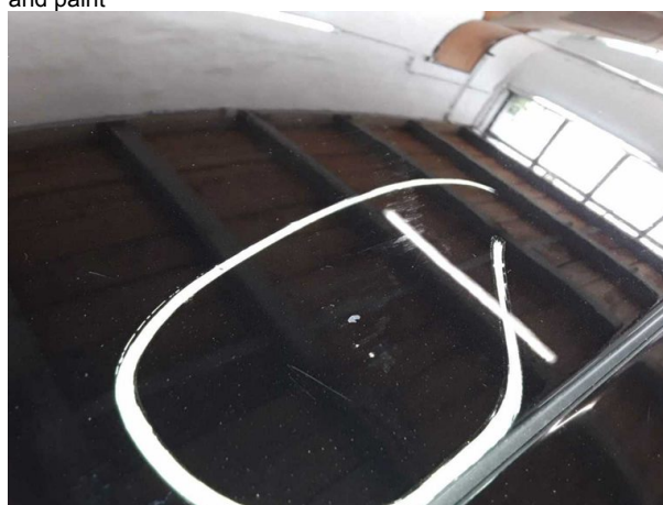
Damage #11: Roof: Roof - Dent / paintcoat damage - Repair and paint
