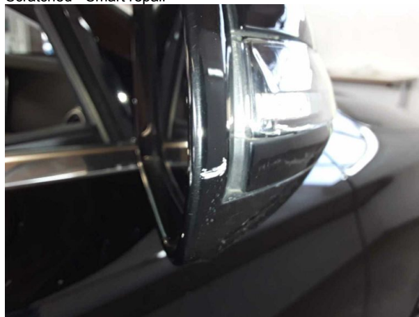
Damage #6: Wing mirror - right side: Mirror housing - Scratch... - Smart repair
