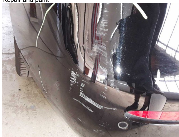
Damage #9: Rear bumper: Bumper with Parktronic - Scratched - Repair and paint
