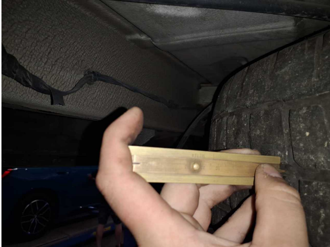
Damage 3: Wheel / tyres: Spare wheel - Worn - Replace
