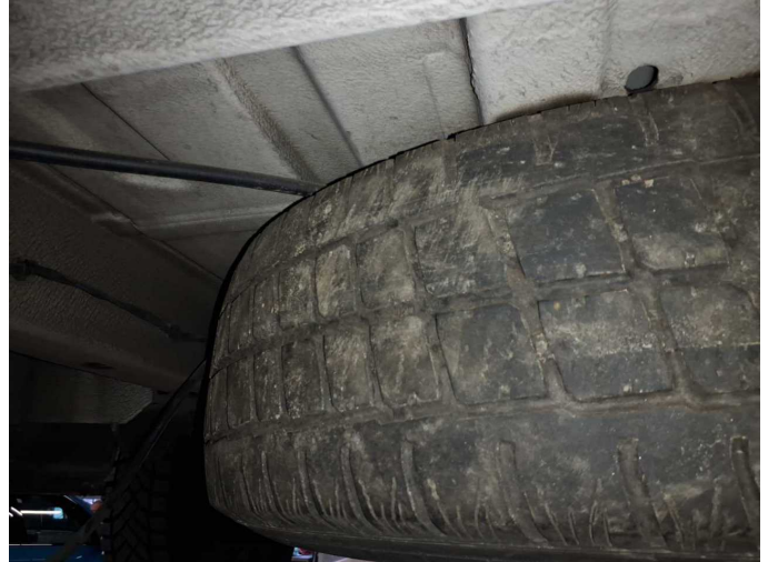
Damage 3: Wheel / tyres: Spare wheel - Worn - Replace
