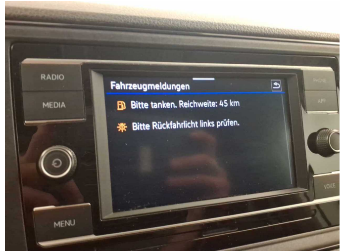
Damage 1: Electrical system: Lighting system - on - Perform diagnosis
