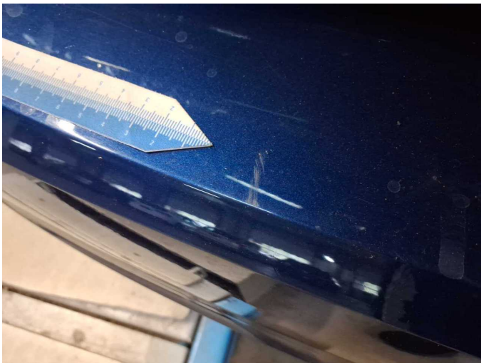
Damage 9: Rear bumper: Rear bumper - Scratched - Paint
