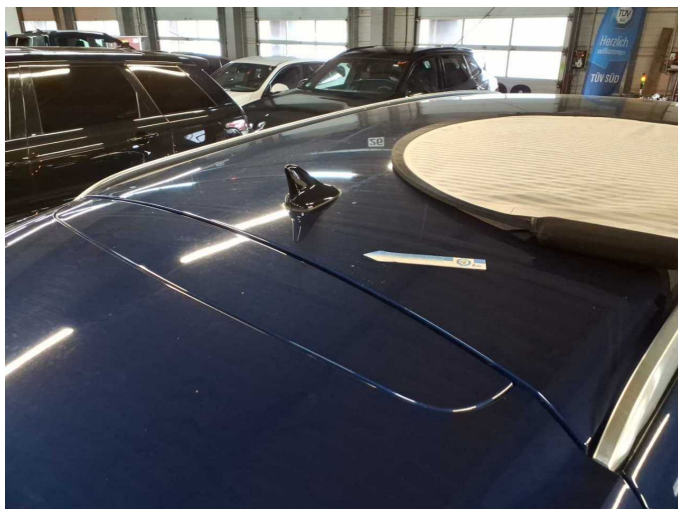
Damage 3: Roof: Roof - dent(s) - Smart repair
