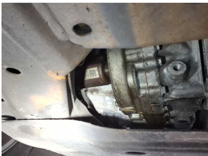
Damage 1: Gearbox: Gearbox - Leaking - Perform diagnosis
