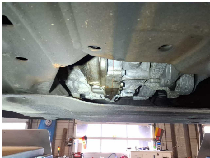
Damage 1: Gearbox: Gearbox - Leaking - Perform diagnosis
