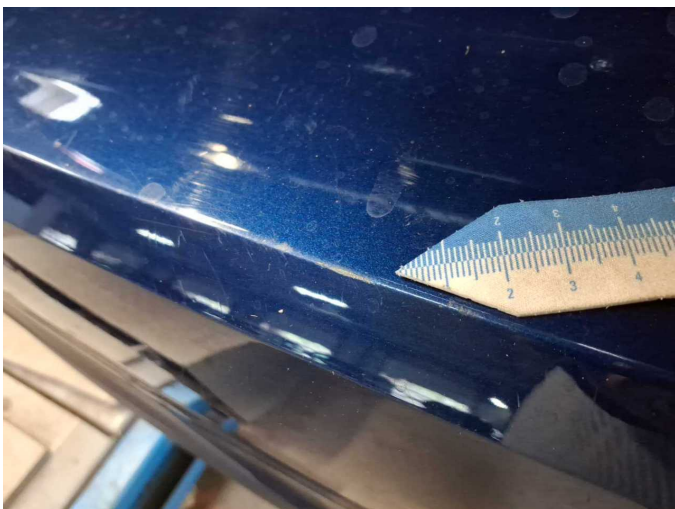
Damage 9: Rear bumper: Rear bumper - Scratched - Paint
