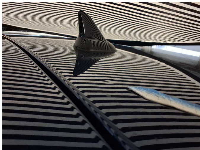
Damage 3: Roof: Roof - dent(s) - Smart repair
