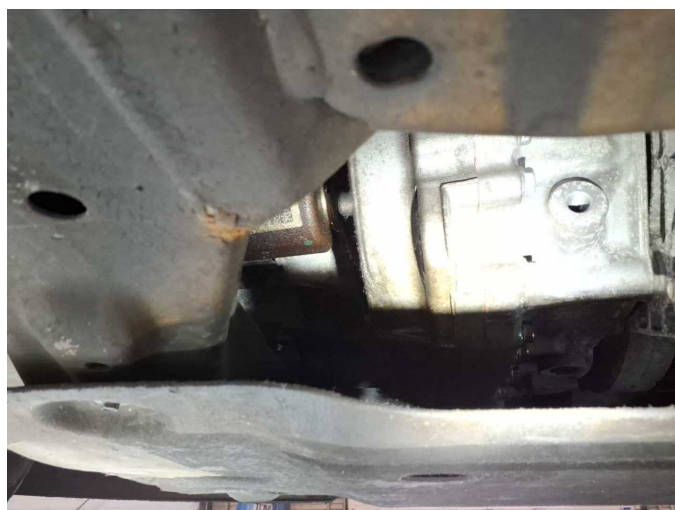
Damage 1: Gearbox: Gearbox - Leaking - Perform diagnosis
