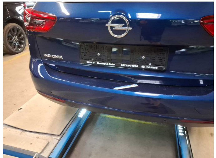
Damage 9: Rear bumper: Rear bumper - Scratched - Paint
