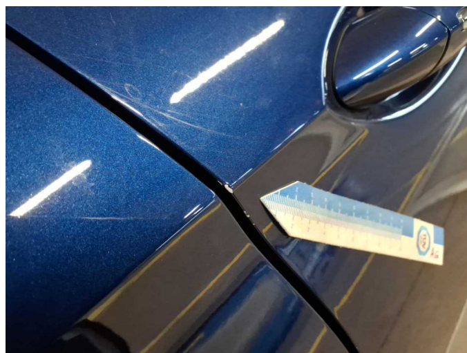
Damage 5: Door - front right side: Door edge - Scratch(es) - Smart repair
