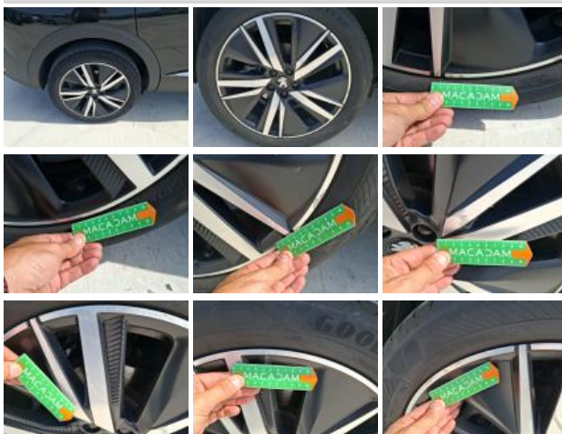
Tyre RR, Tear, Replace
