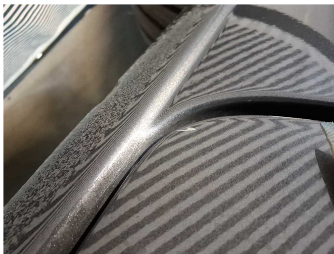
Damage 16: Sliding door, right: Sliding door (Delle) - Scratched - Repair and paint
