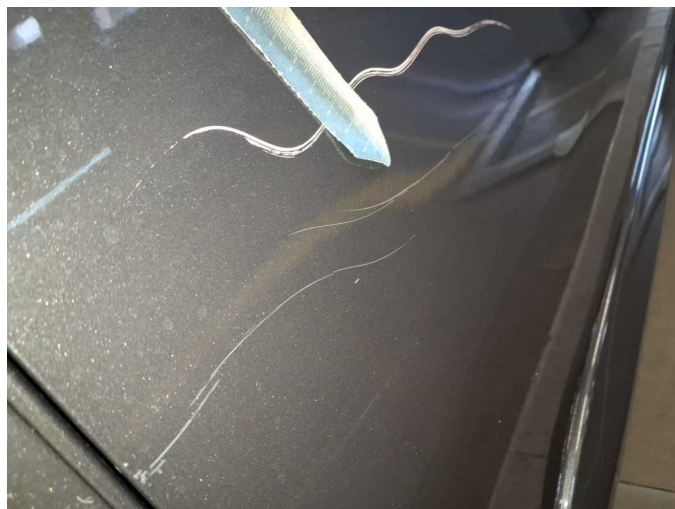
Damage 16: Sliding door, right: Sliding door (Delle) - Scratched - Repair and paint
