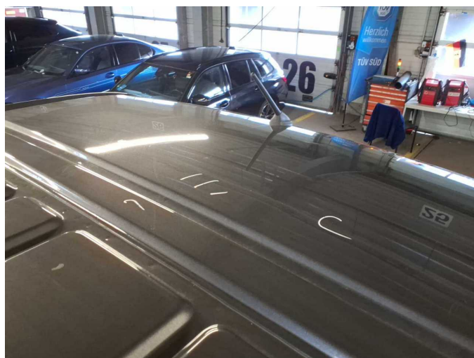
Damage 6: Roof: Roof (vorne) - dent(s) - Smooth repair work
