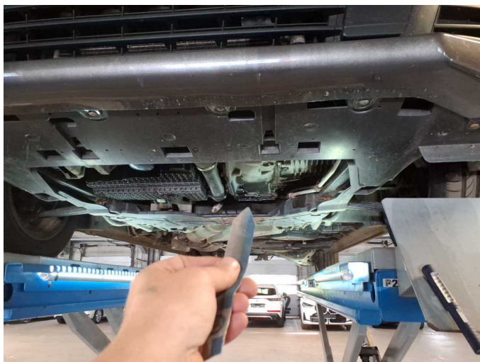
Damage 1: Gearbox: Gearbox (Tröpfchenbildung, Umweltbelastung) - Leaking - Perform diagnosis
