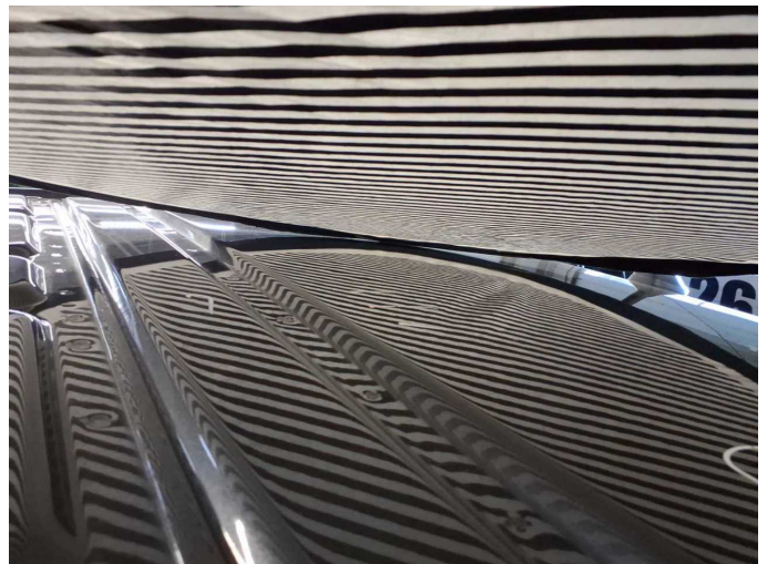
Damage 18: Roof: Roof (Mitte) - Dent / paintcoat damage - Repair and paint
