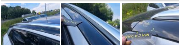
Door RR, Dent(s), Paintless dent repair
