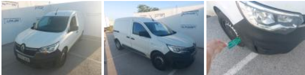
Wing FR, Dent(s), Repair and paint (complete)
