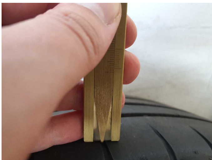
Damage 6: 2nd wheel set: 3 tyres - Worn - Replace
