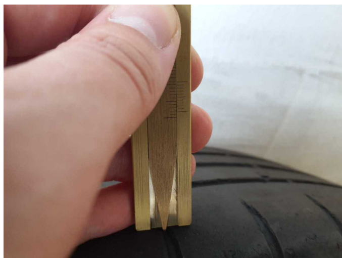
Damage 6: 2nd wheel set: 3 tyres - Worn - Replace
