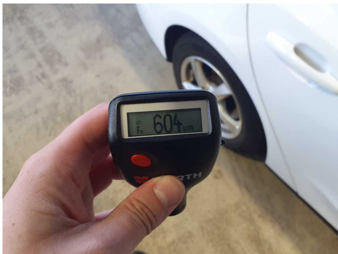
Repainting 3: Side panel - rear right side
