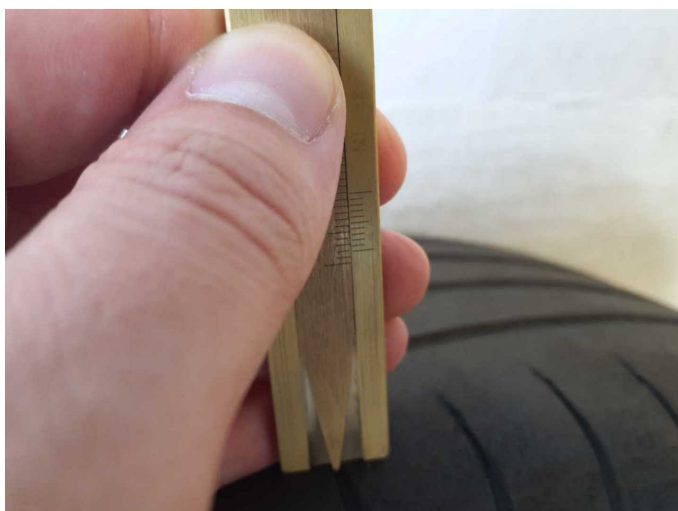
Damage 6: 2nd wheel set: 3 tyres - Worn - Replace
