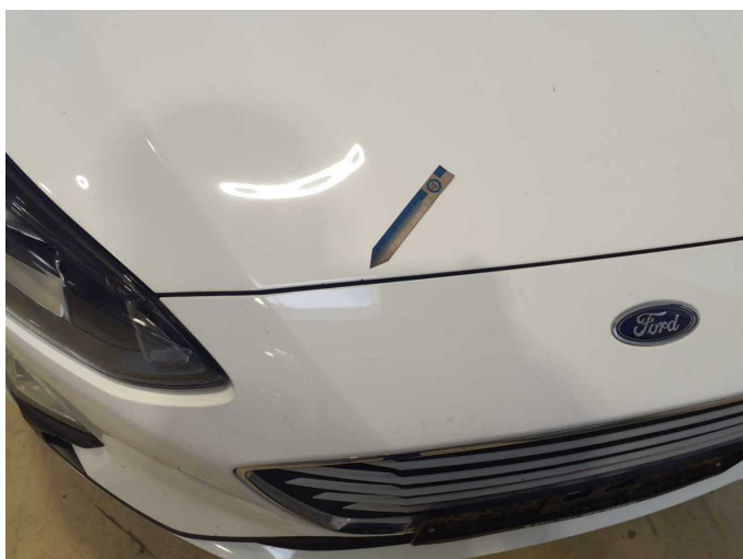
Damage 9: Bonnet: Bonnet - Corrosion - Repair and paint
