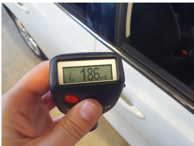
Repainting 1: Roof rail - right side
