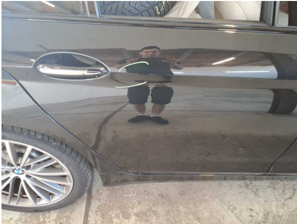
Damage #2: Door - rear right side: Door - Scratched - Loss in value
